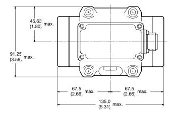
Torque mounting screws to 9 to 14 Nm (80 to 120 lb.in.).
